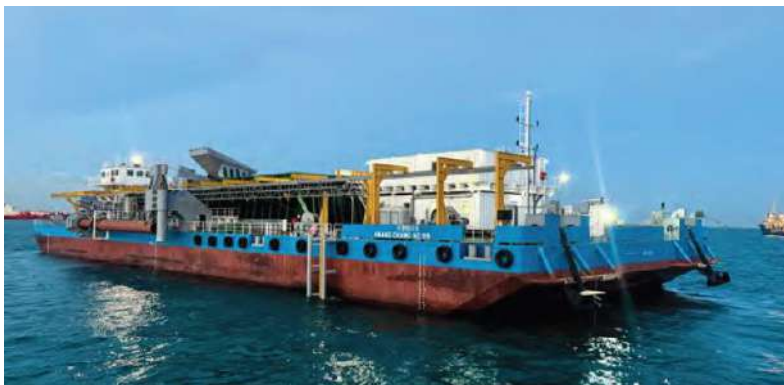
Subsea Rock Installation Barge Sea Trials
