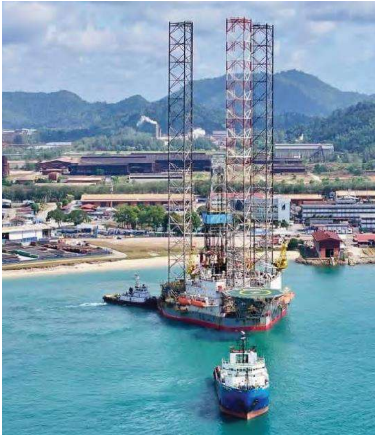
Bridgewater 168: Jack-Up Rig Towage Operations
